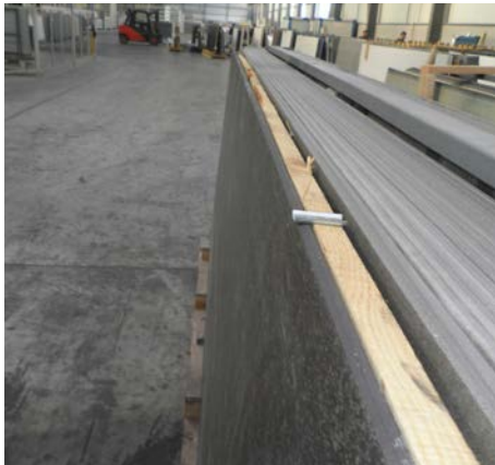
Image 3: Plank in the backside of the slab
